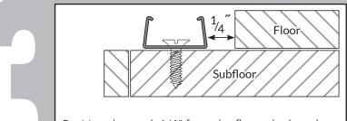
Position the track 1/4" from the floor plank and screw to the subfloor using included screws.
