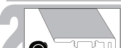
Install the flooring leaving a 1-1/4" gap between the two floor surfaces for the end cap installation.
